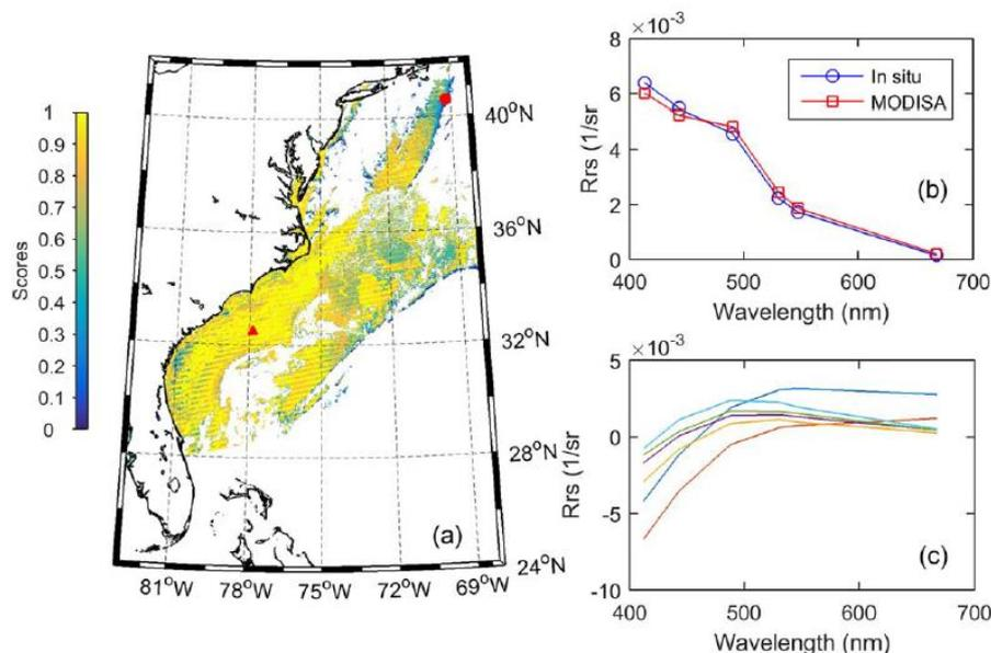
Figure 2. Quality evaluation of the MODISA ocean color data in US East Coasts and the Northwest Atlantic Ocean. (a) Scores of the satellite ocean color data (11 December 2015, A2015345180500.L2\_LAC). (b) Comparison of the satellite ocean color and in situ data measured at a station indicated by “ $\Delta$ ” symbol in Figure 1a (Station number: 20; position: 32.49448N,
