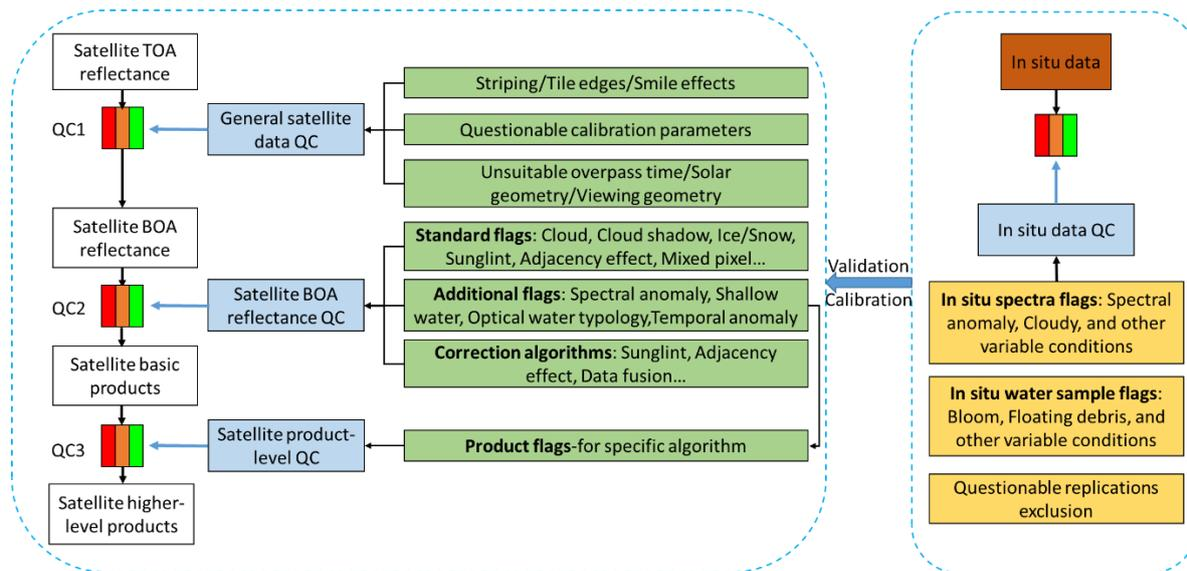
Figure 1. Framework of Quality Control (QC) procedures throughout the process of CoastObs EO products. Three colours represent three types of reliability of the data to a specific indicator (Green represents good, amber represents warning, and red represents fail.)
