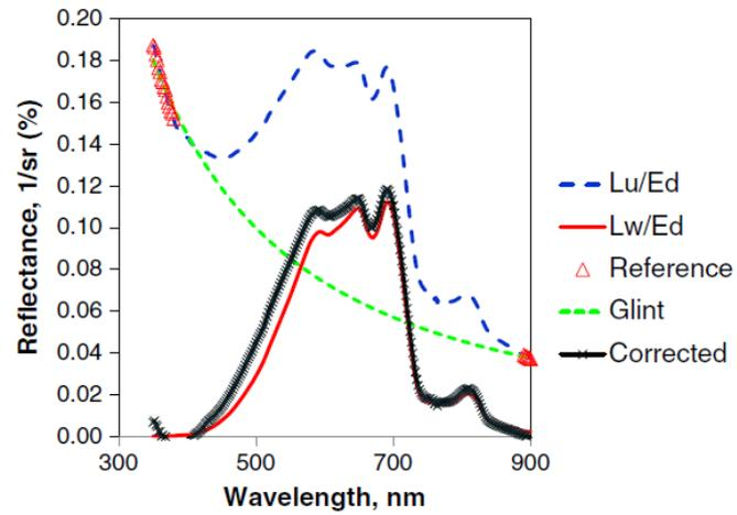
Figure 6. Results of the reflectance measurements carried out in Lake Peipsi on May 12, 2011. The measurements were carried out in optically deep water in optimal conditions (around noon, nearly clear sky, calm). “ $L_u/E_d$ ” is an average reflectance spectrum measured above the water surface; “ $L_w/E_d$ ” is an average remote sensing reflectance spectrum measured with the black tube of radiance sensor just below the water surface (Kutser et al., 2013).
